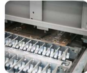
Recovery glass(Ag) on PDP panel by automatic equipment
