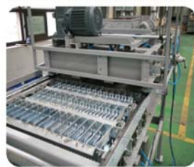
Recovery glass(Ag) on PDP panel by automatic equipment
