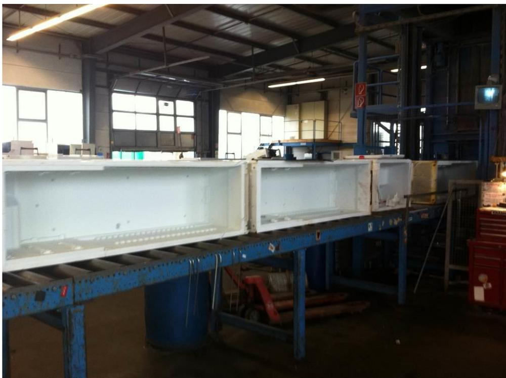
All other appliances were sluiced in between the Step 1 and Step 2 plants and fed to the appliance loading. A door, also with VIP, was added to approximately 80% of appliances. Packages of 3 to 4 doors were assembled and added to every four to five appliances. The plant throughput was approximately 30 appliances per hour.
