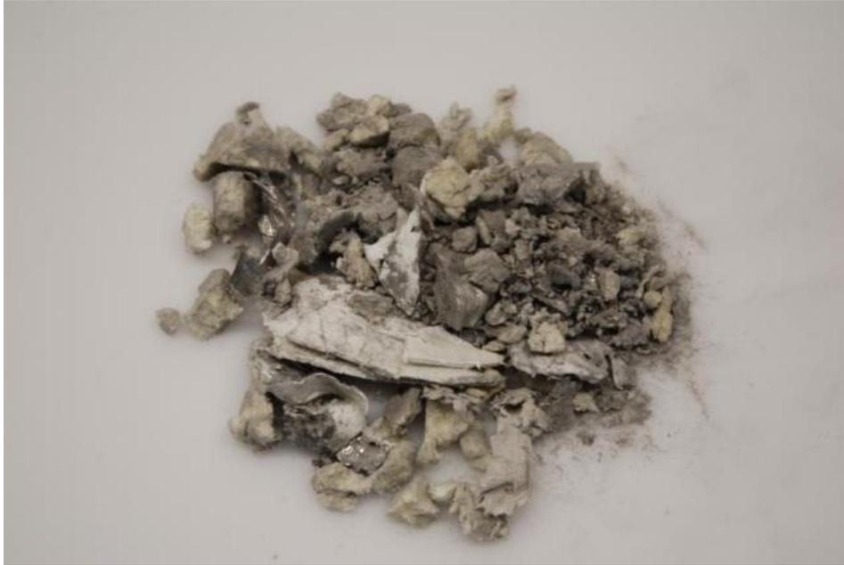
Sample 3 after 20 to 25 refrigeration appliances with VIP. Sample taken at: screw conveyor after pre-shredder
