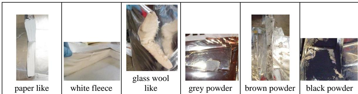
Figure 1: Different Material Groups of the Vacuum Insulation Panels
