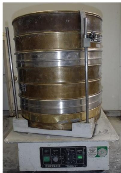
Figure 6: Sieve Tower on Mechanical Shaker
