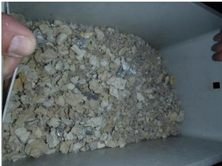
Figure 18: PU Output Mixed Up with VIPs’ Material
