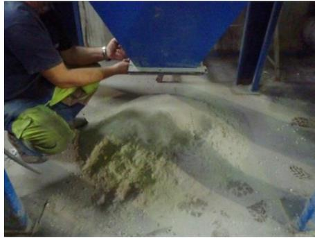
Figure 41: Residue on the Filter directly behind the Shredder
