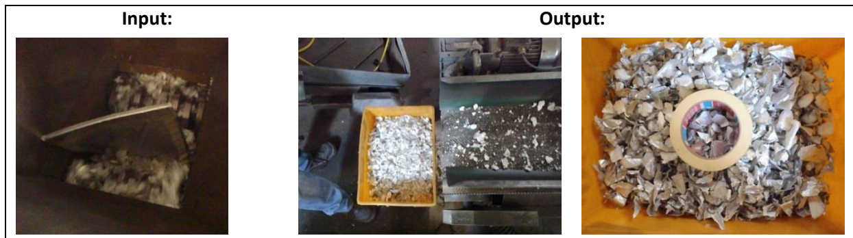
Figure 28: Input and Output Material of Material Group 1 (paperlike)
