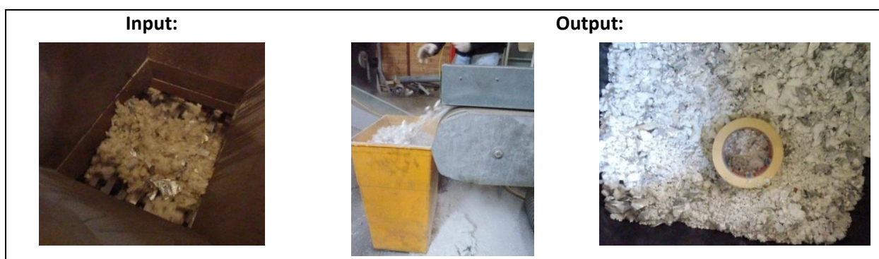
Figure 30: Input and Output Material of Material Group 2 (white fleece)
