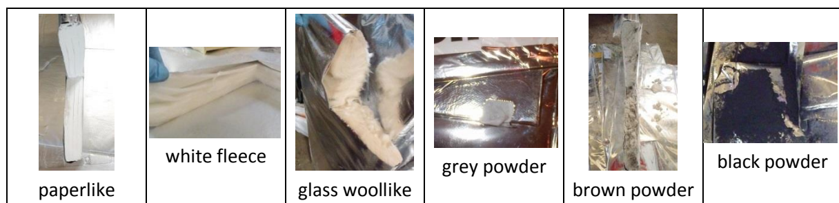
Figure 5: Different Material Groups of the Vacuum Insulation Panels
