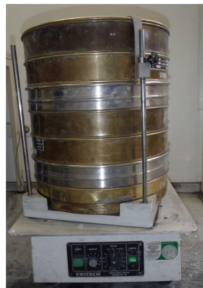
Figure 35: Sieve Tower on Mechanical Shaker
