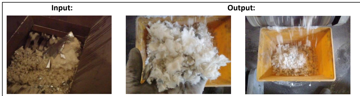
Figure 31: Input and Output of Material Group 3 (glass woollike)
