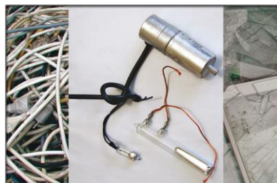
Fig. 5.46 Fractions removed, e.g. cables, mercury switches
