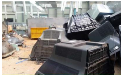
Fig 5.27 Back-cover removal & Funnel cutting
