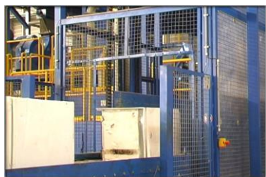
Fig. 5.49 Sealed shredding through air lock gates
